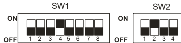
Figure 2: Switch Settings for Diamond I/O Module 200
