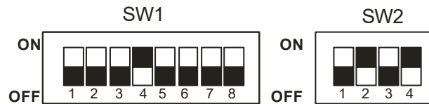
Figure 3: Strap and Switch Settings to allow Diamond I/O Module 200 to be DFR Clock Source
